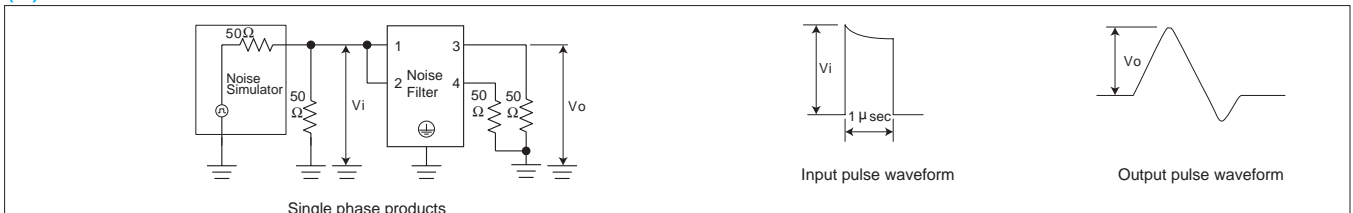
Fig.3.7 Pulse attenuation measurement diagram
