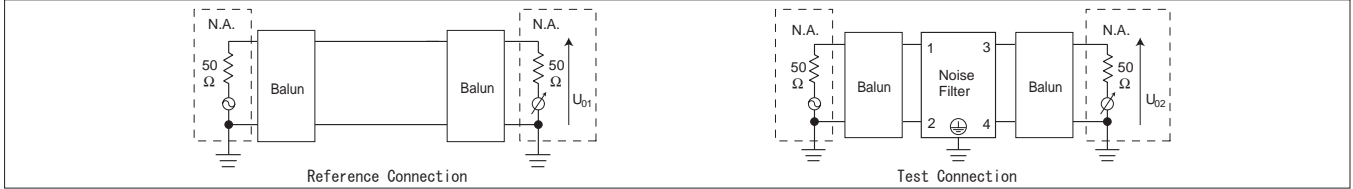
Fig.3.1 Differential mode attenuation measurement diagram
