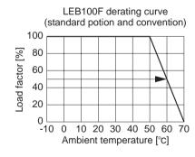
Calculating A<sub>1</sub>, A<sub>2</sub>, A<sub>3</sub> A1=I01/I1×100=0.2/5×100=4  $A_2=I_{02}/I_2\times 100 = 2/4\times 100 = 50$ A3=(V1xlo1+V2xlo2)/(TOTAL OUTPUT WATTAGE)x100  $=(5\times0.2+24\times2)/100\times100=49$
