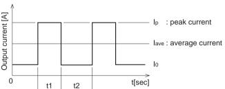
t1  $\leq$  10 [sec], lave =  $\frac{l_p t_1 + l_0 t_2}{t_1 + t_2} \leq$  rated current,  $\frac{t_1}{t_1 + t_2} \leq$  0.35
