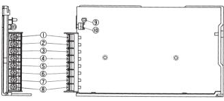
①V1 Output ②G1(V1)GND ③V2 Output ④G1(V2)GND ⑤NC ⑥Frame ground
